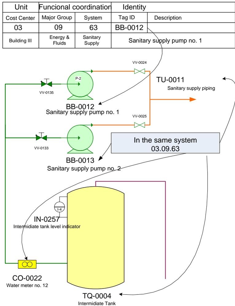
Fig. 1 – Coordination and coding of a maintenance item in a building
